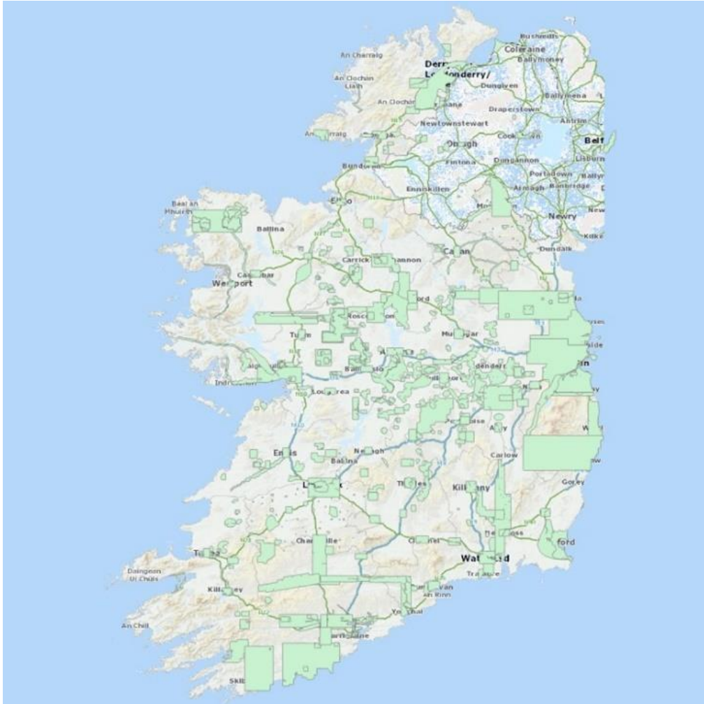
Figure 13: Overview of available point cloud datasets in Ireland, where in green the regions with available LiDAR point cloud data are available (Tailte Éireann, 2025)
