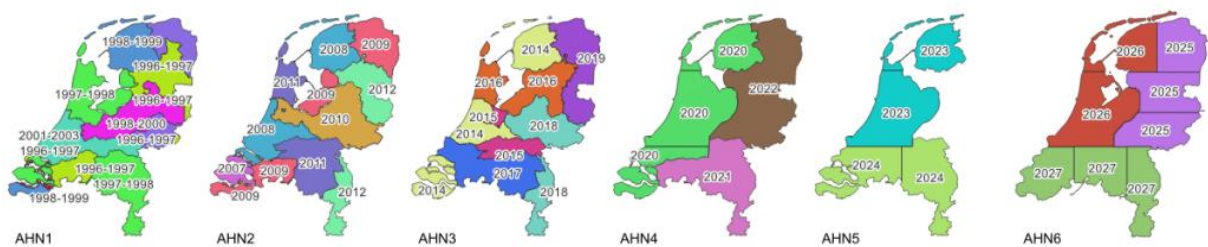
Figure 15: Acquisition cycles in the Netherlands' national point cloud dataset (AHN1 to AHN6).
