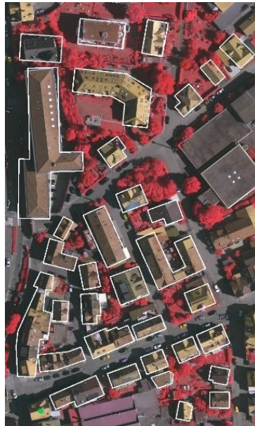
Figure 28: Generated vector data of buildings superimposed onto the DSM-based ortho-image. The green dot marks an undetected building. (Source: Höhle, 2021)
