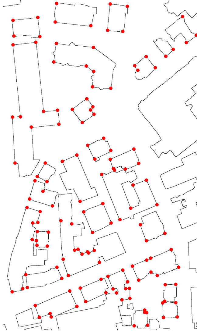
Figure 19: Distribution of checkpoints along with the buildings extracted from a manually compiled land cover map (ISPRS data set, area #1). (Source: Höhle, 2021)
