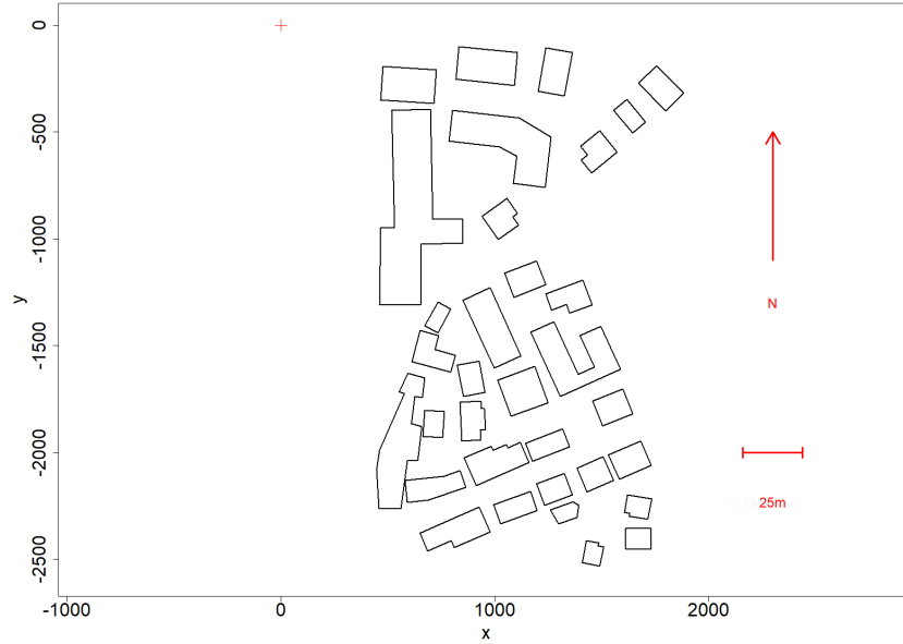
Figure 27: Vector data derived from a DSM-based orthoimage by the software package “buildenh”. (Source: Höhle, 2021)
