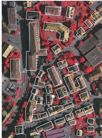
Figure 18: Enhanced outlines of buildings plotted on top of an DSM-based orthoimage. (Source: H hle, 2021)
