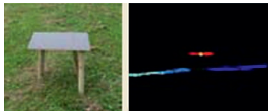
Figure 4.3 Ground control and checking in corridor projects using ALS. Targets with elevation difference to the ground and special reflecting material (left) can precisely be identified in the dense point cloud (right). Source: Flatman 2009
