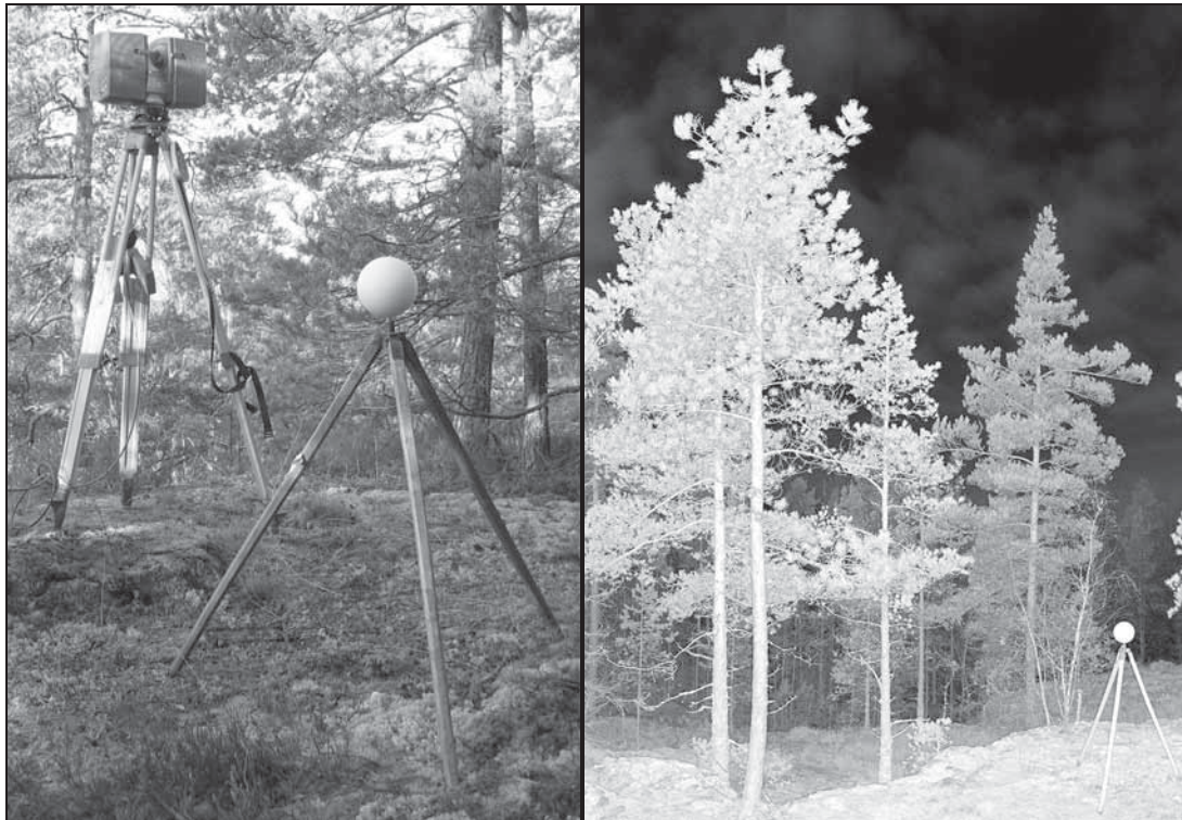
Figure 2-2: Terrestrial laser scanner and spherical reference target on the left, on the right part of a scanned point cloud illustrated as planar intensity image.
