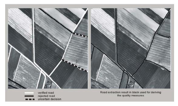
Figure 4: The result of the fully automatic quality control of the verification step as it is transferred to the interactive quality control by an operator.
