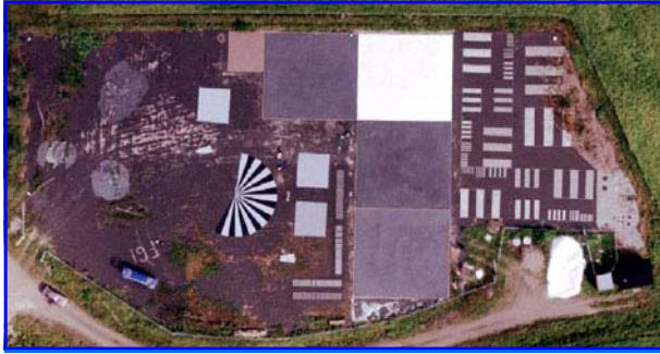
Figure 2. New geometrical resolution and reflectance reference targets in the FGI Sjökölla airborne sensor systems test site
