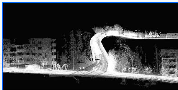
Point cloud obtained with FGI-built ROAMER system.
