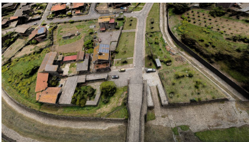
Exemplary 3D point cloud obtained with a traditional approach for 3D reconstruction from imagery
