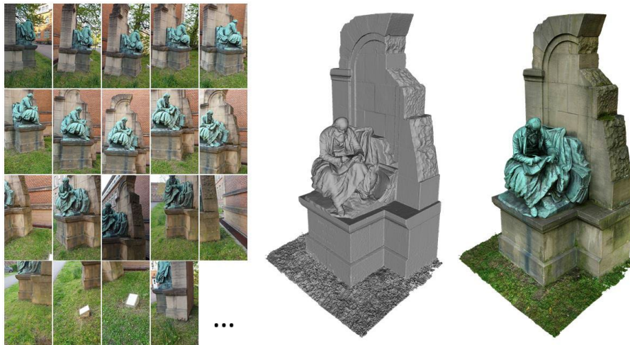
3D reconstruction from imagery: given a set of input images (left), the main objective is to derive a 3D scene representation in terms of geometry and colour information
