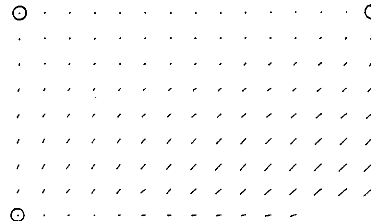
FIGURE 8 DISCREPANCIES WITH 3 CONTROL POINTS (CIRCLED) - RMSE=1.6mm
