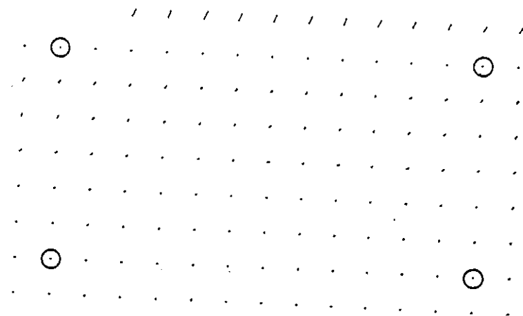
FIGURE 11 DISCREPANCIES WITH 5 CONTROL POINTS (CIRCLED) - rmse = 0.4mm
