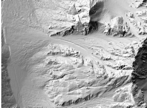
Fig. 6. Shaded digital surface model, derived from all ALS points. Rocky terrain with relatively little vegetation is visible. Project of the “Landesvermessung Vorarlberg”.
