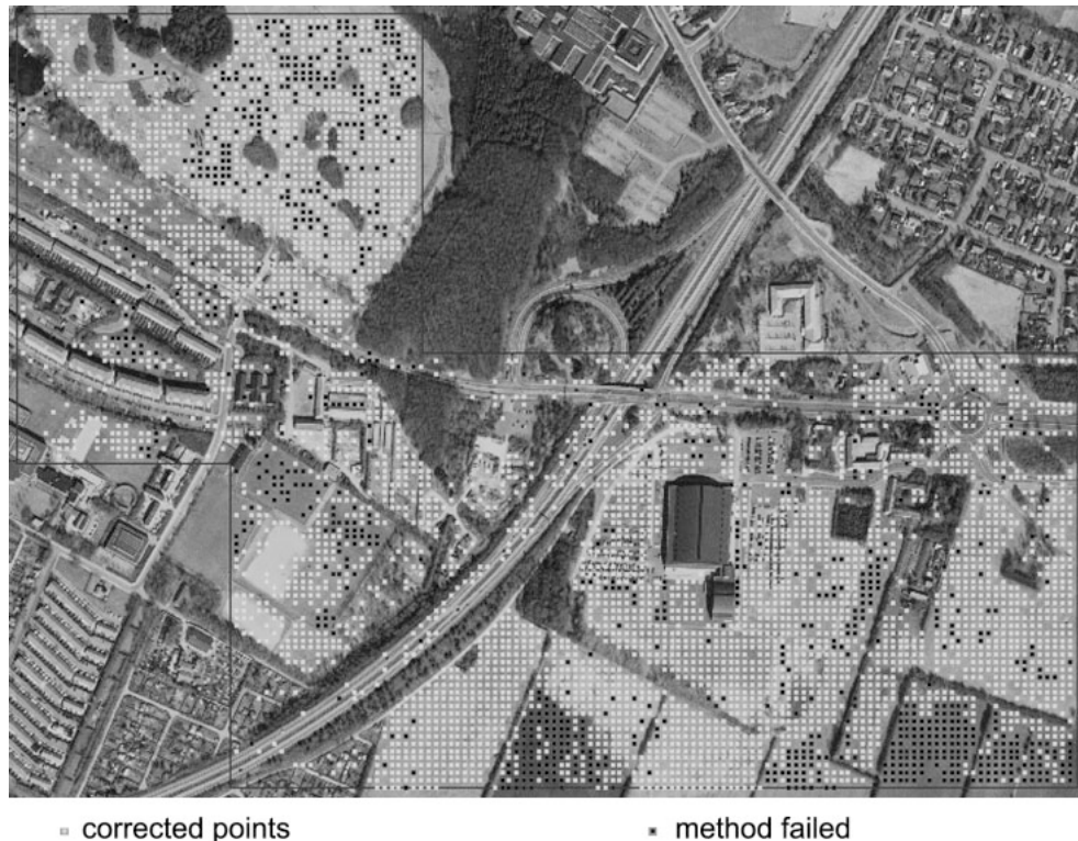
Fig. 3 Division of the tested DTMs into two categories, example of Test B, subarea A_I. White (green) points fulfilled all set criteria and comprise a minimum of blunders, dark (red) points must be checked by other methods. The distance between points is 10 m.
