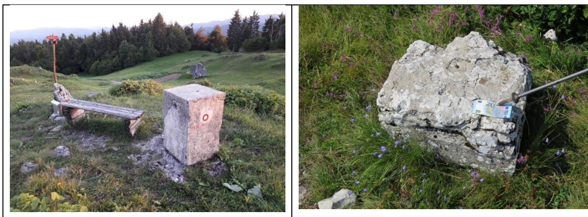
Figure 1: Different types of markers for trigonometric points based on the institution that made its stabilisation in the past.
