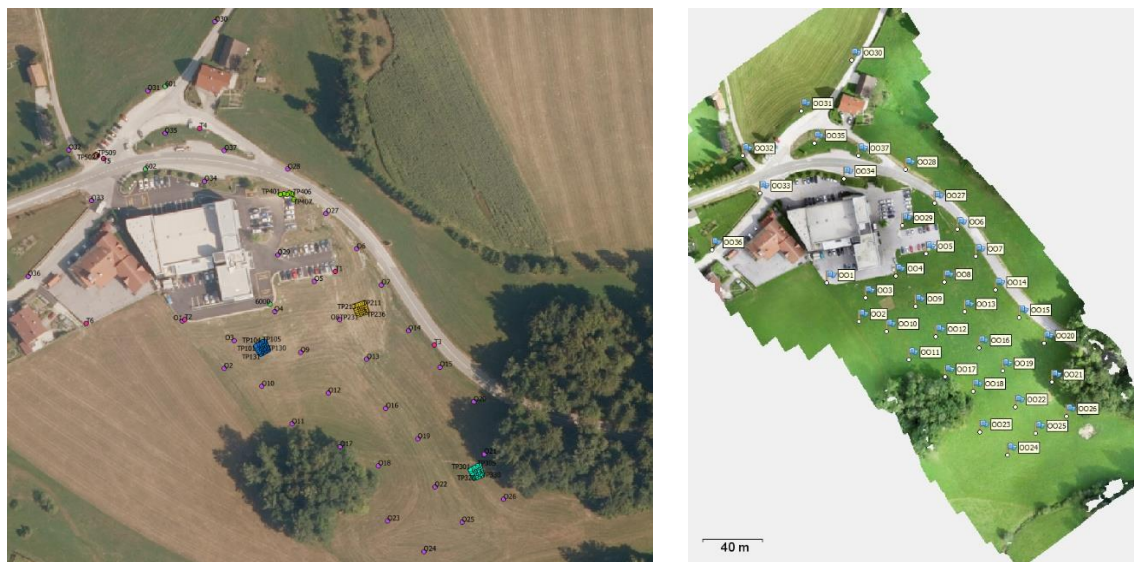
Figure 2: The study area of Kandrše with the network of grounds control points and »test fields with targets (left) and UAV photogrammetric cloud with labelled control points (right).
