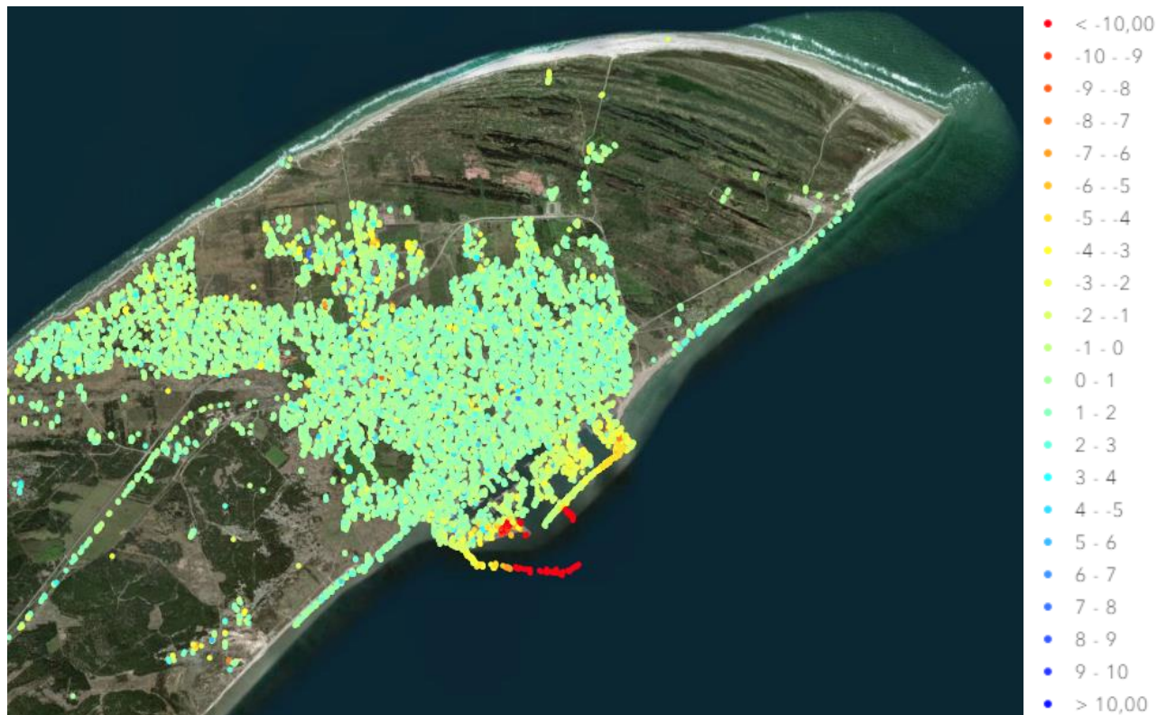
Figure 1. Deformations over the town Skagen in Northwestern Denmark, given in mm/yr. Red shows movement away from the satellite and blue movement towards the satellite. The movement of most infrastructure is resolved: The main road leading to Skagen, buildings, the rock dikes along the coast, the infrastructure on the port, etc. For example, a great subsidence is seen by the port resulting from construction works. Courtesy: TRE Altamira (2020). This work contains modified Copernicus Sentinel data 2014-2019.
