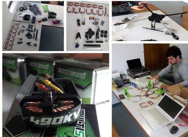
Figure 5: Building the quadrocopter from the purchased components ( http://www.geodetski-vestnik.com/58/3/gv58-3_dougan.pdf )
