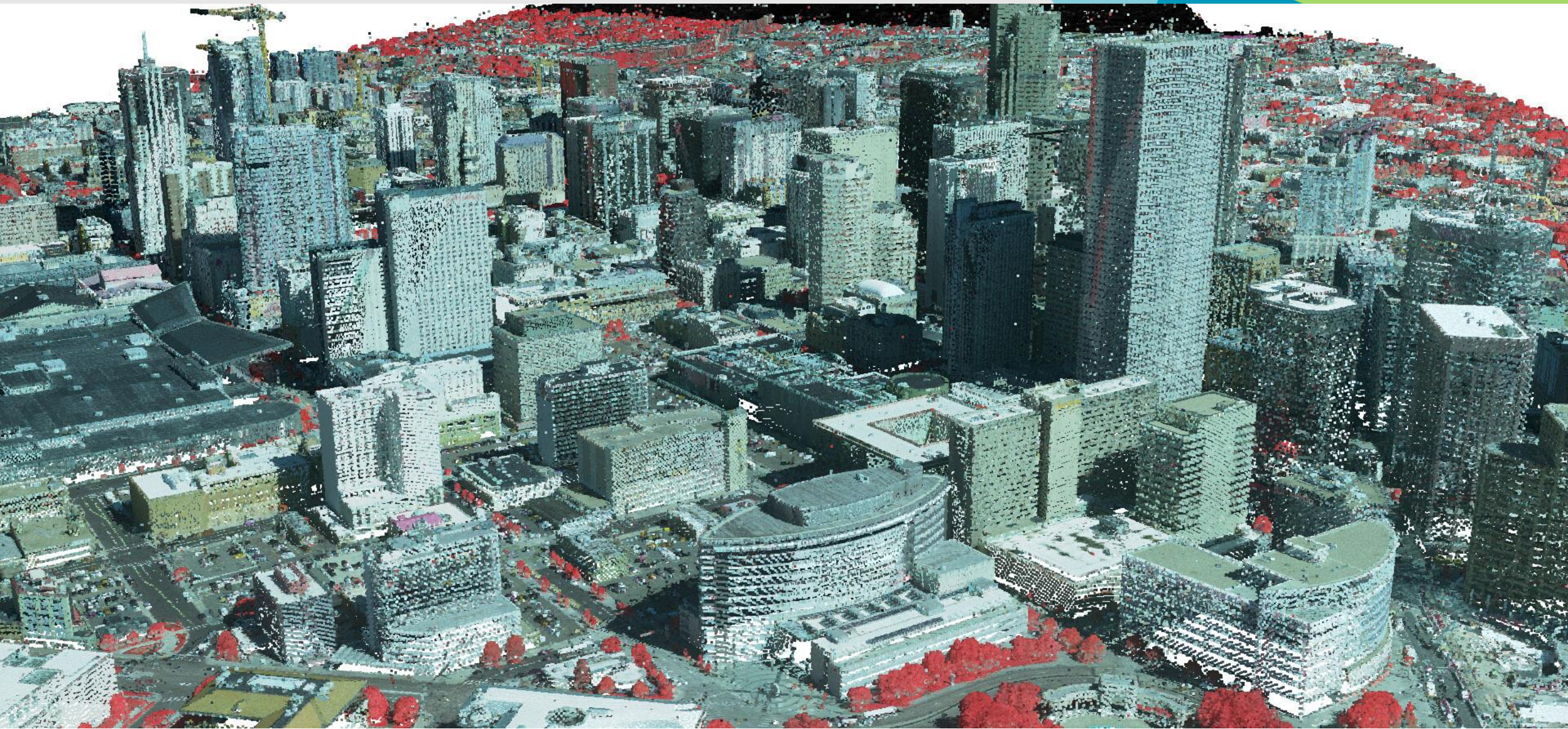
Frankfurt city center generated by BuildingFinder, data source TerrainMapper LiDAR sensor
